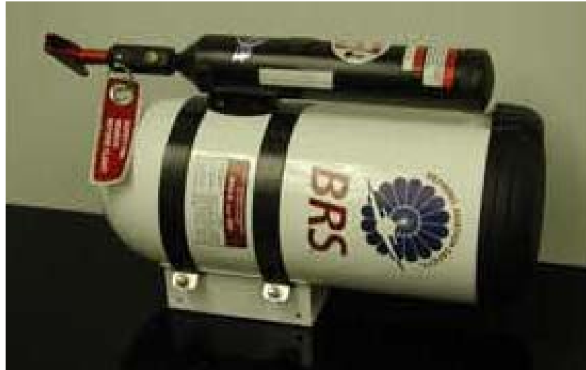
Fig. 6: Parachute packed in canister
