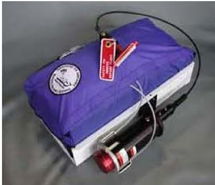
Fig. 8: Parachute packed in bag with Velcro seal
