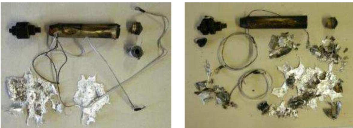
Fig. 6: FCO results for the BRS 440 respectively for test V01 (left) and test V03 (right).
